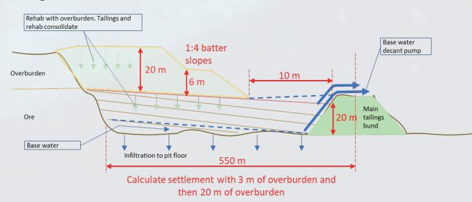
Above: Start of cell rehabilitation with the initial level of overburden above the original ground level to allow for consolidation as settlement of the tailings increases under their own weight.
