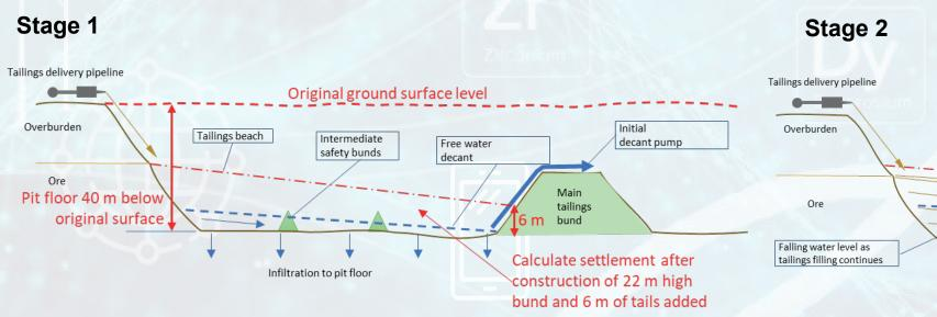
Above: Start of tailings deposition, when they are fully saturated, after bund construction.
