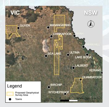
The aircraft will fly at a nominal ground clearance of 35-50 metres rising up to 300 metres above townships and houses. Flying will occur only during the day and only in favourable weather conditions. The survey will not involve any ground disturbance.
