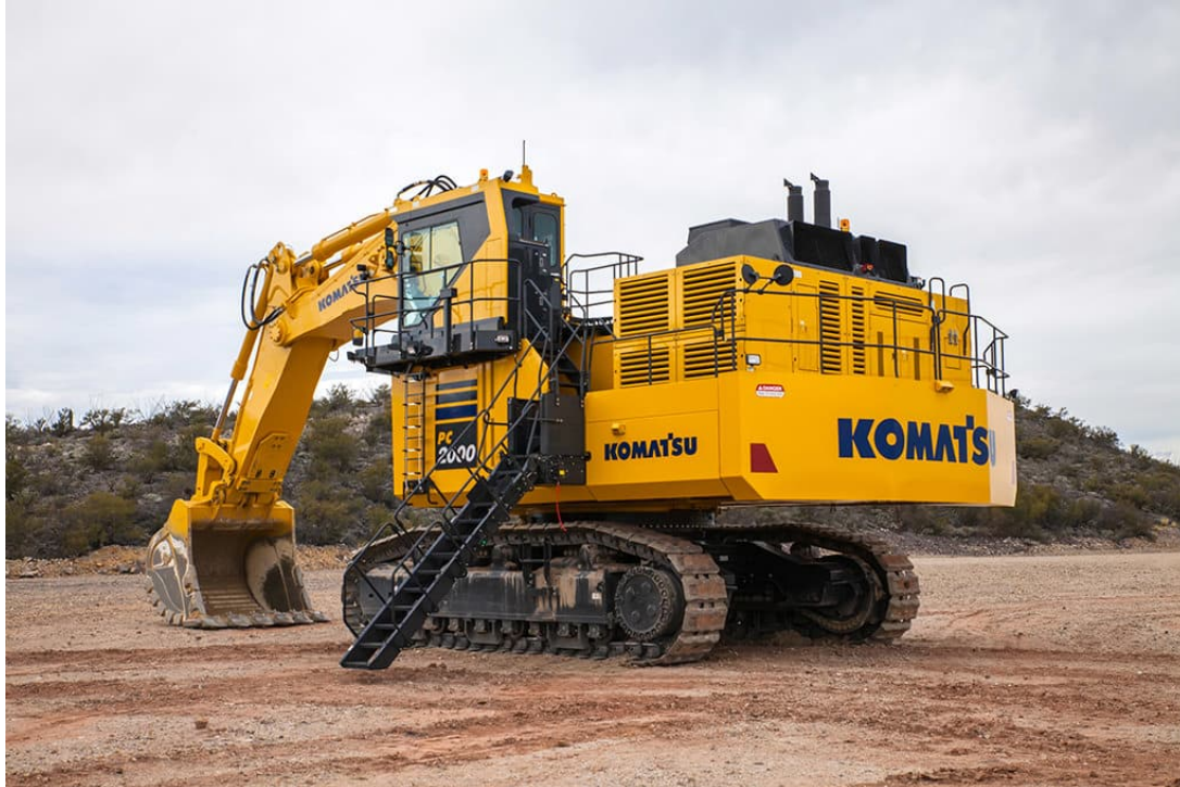
Photograph 3-1 200 tonne excavator (Source: Lectura specs)
