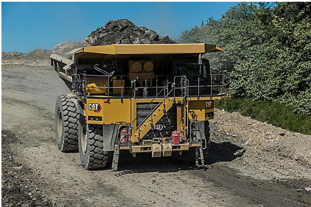
Photograph 3-2 A 130 tonne rigid body truck (Source: Cat)
