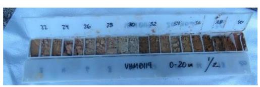
Figure 14: Photograph of representative samples retained from exploration drilling
