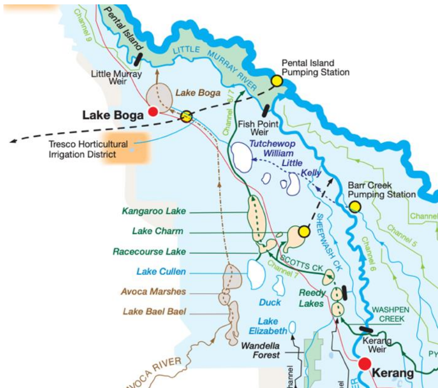
Figure 3 Schematic Representation of the Kangaroo lake portion of the Torrumbarry Irrigation System (Source: NCCMA)
